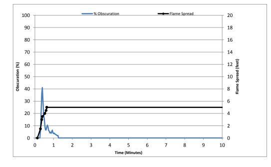
Test Num.: 3 MH61932 / 4787671596 12171605 Flame Spread Index: 25 Smoke Developed Index: 10
