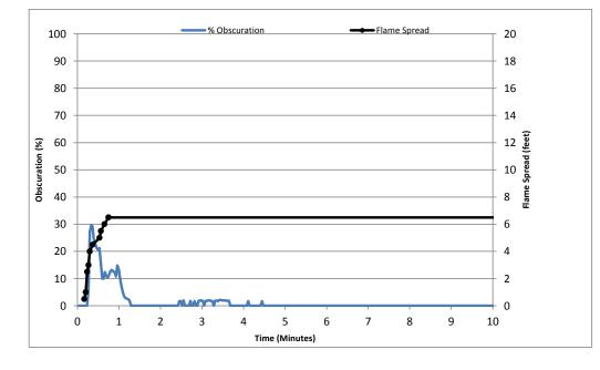
Test Num.: 4 MH61932 / 4787671596 12171606 Flame Spread Index: 30 Smoke Developed Index: 20
