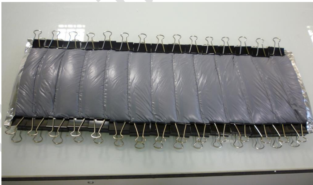
Figure 1 : Test specimen of ISOAFS-VINYL ECOSOFT ventilation duct (internal face)
