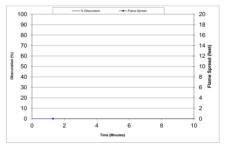
Test Num.: 2 MH48069 / 11CA08190 04081109 Flame Spread Index: 0 Smoke Developed Index: 0
