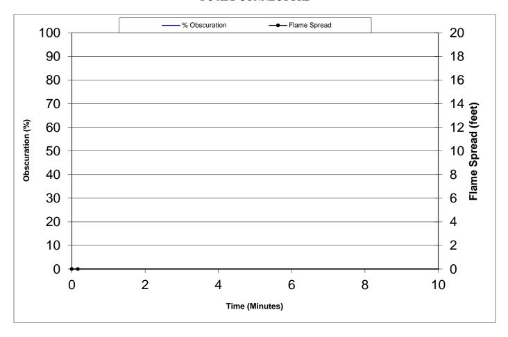
Test Num.: 1 MH48069 / 11CA08190 04081107 Flame Spread Index: 0 Smoke Developed Index: 0
